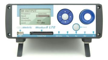
This capability includes RF channel emulation allowing the tester to generate a RF signal as seen at the output of the base station transmit antenna or the input from a handsets receive antenna. Both transmit and receive Multi Input Multi Output (MIMO) antenna configurations can also be emulated by using two synchronised Modus 6 air interfaces.
