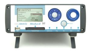
RF output can be in the range 100MHz to 2.2GHz in a continuous range with levels between 0dBm and -110 dBm in 0.5dB steps, set using the internal electronic attenuator.
