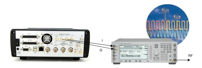
Modus 4 has differential I/Q analogue base band RF outputs which can be used to drive a external I/Q Vector Signal Generator like the Agilent ESG-C to provide a reference quality RF output with 0.1db resolution and very low phase noise. The I/Q outputs from the Modus 4 are of 16 bit resolution and are the same I/Q data used internally by the Modus 4 up converter stage.
