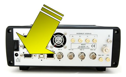
Modus 4 can be upgraded remotely using the 9 way RS232 port on its rear panel. Upgrade instructions are as follows:
